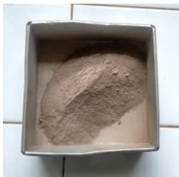
Figure 1. Sedimentary Soil from Bili-Bili Dam
